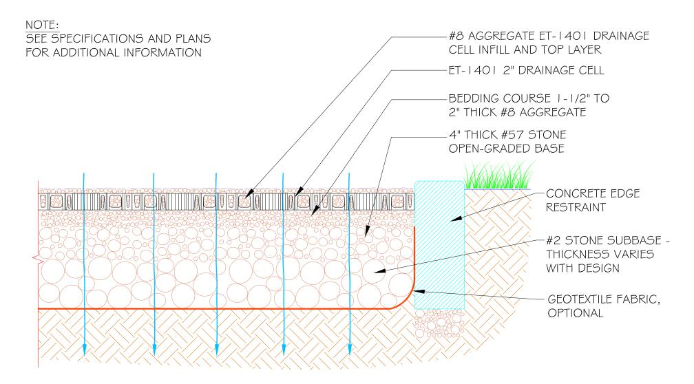
CONCEPT DRAINAGE CELL GRAVEL PAVER INSTALLATION SECTION - FULL EXFILTRATION
